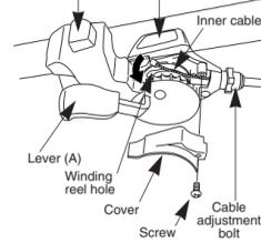
While firmly pulling the inner cable, secure by tightening the fixing bolt with a 5 mm Allen key.
