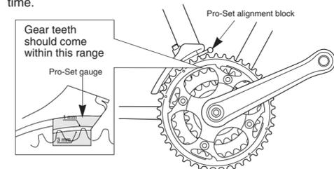
The level section of the chain guide outer plate should be directly above and parallel to the largest chainring. Secure using a 5 mm Allen key.
